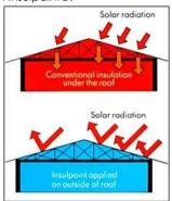
The diagram on the right shows results for Insulpaint® when compared against the other conventional insulating systems.
