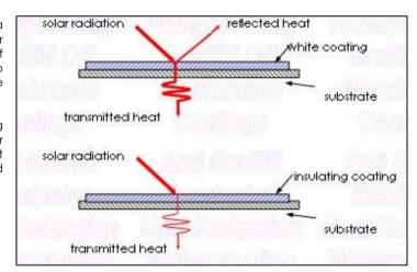
The diagram below shows how a light coloured insulating coating would behave if shown diagrammatically. It can be seen that some of the solar radiation is reflected and the remaining heat load is reduced because of the thermal barrier providing by the insulating coating.
