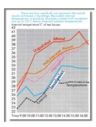
This result was far better than both the fibreglass and polystyrene foam insulating systems.
